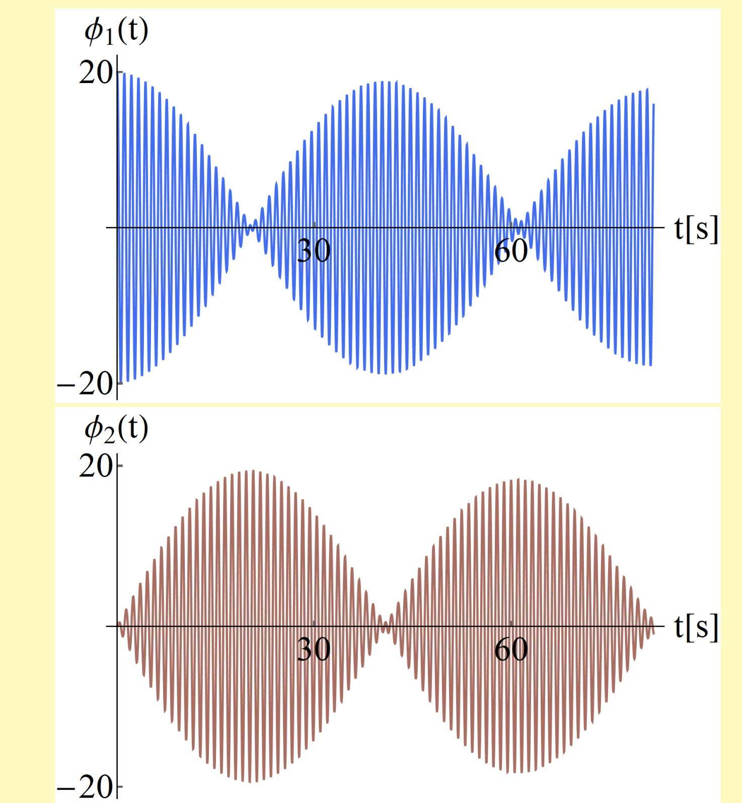
For sufficiently large times, anti-phase synchronization between the two pendula occurs.
