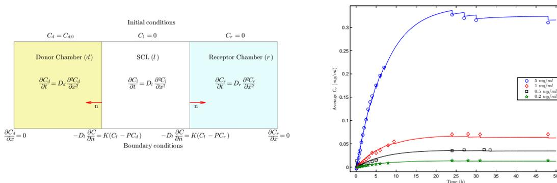
Figure 1: Left: Schematic of experimental system. Right: Release profiles compared with experimental data.
