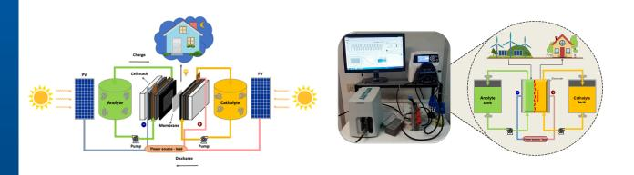
Conversion of solar radiation into electrochemical energy with a redox flow battery (RFB) replacing vanadium (inorganic) with allorganic active compounds | Fully organic solar powered redox flow battery prototype and proof of concept from University of Coimbra
