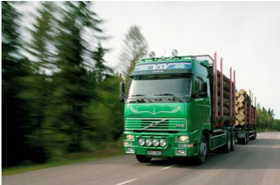
Figure 1: Transport vehicles are exposed to dramatically different conditions in different parts of the world and different transport missions. The timber truck needs to sustain very high payload loads, as well as high dynamic loads.
