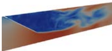
Figure 1: Simulation of the turbulent flow of air past a mixer plate in an exhaust system (simulations by Rodrigo Vilela De Abreu and Johan Jansson at CTL).
