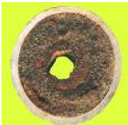
Section of a pipeline with deposited wax
